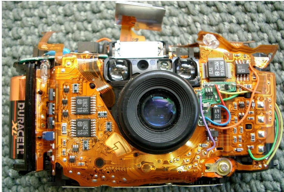
Figure 3-17: Flex Circuit Example; An image containing an example implementation of a flex circuit; reprinted with permission from Steve Jurveston
