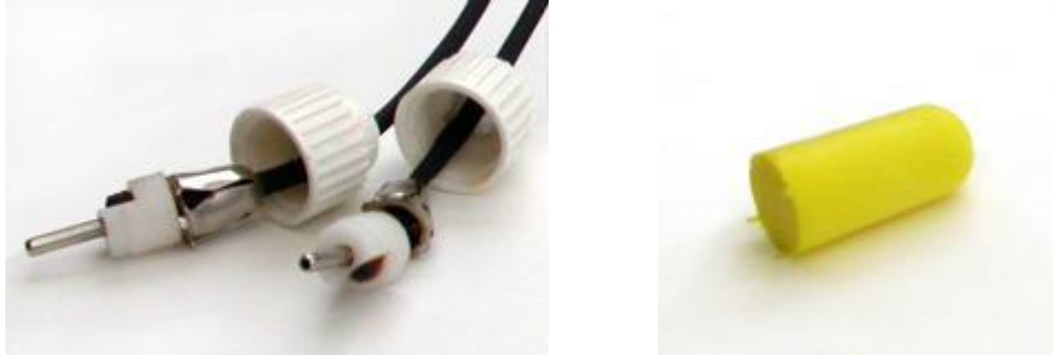
Figure 3-6: DIY Electrodes; An image showing the building process on a DIY electrode; reprinted with permission from OpenEEG
